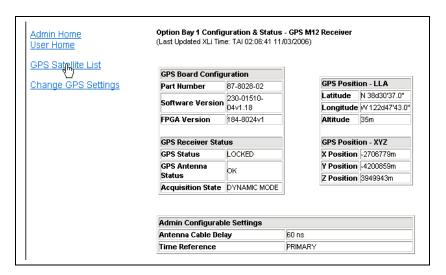
5. (Optional) While waiting for *GPS Status* = *Locked*, click the link for **GPS Satellite List**. The *Tracked Satellite List* must show at least four "Current" satellites for the GPS receiver to initially lock. A low number (<4) of GPS satellites indicates a potential problem with GPS signal strength or visibility at the current site.
